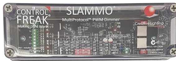
SLAMMO v5 in an IP67 Enclosure
