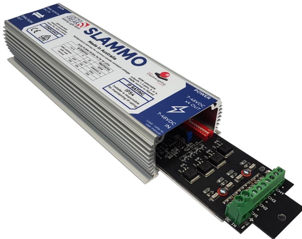
Pictured: SLAMMO in IP54 enclosure – also available as OEM PCB or IP67
